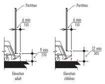
Fig. 11b Vertical Toe Clearance.
