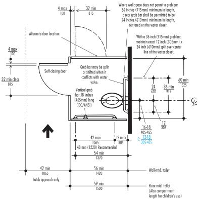
Fig. 9 Large Wheelchair Accessible Toilet Compartment.
