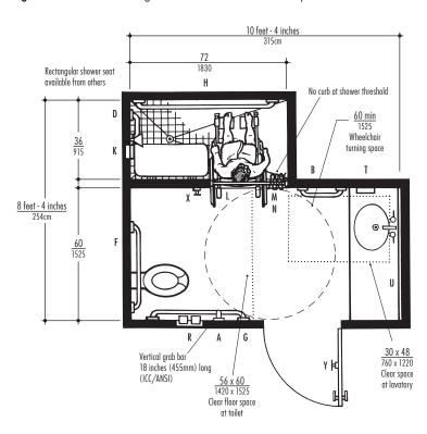
Fig. 32 Bathroom with Combination Tub/Shower Unit and Portable Seat.
