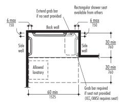
Fig. 24a Standard Roll-In Type Shower Compartment.
