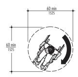
Fig. 2a 60 inch (1525mm) Diameter Turning Space.
