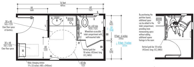
Fig. 18a Accessible Restroom with Additional Entry Clearance Space.
