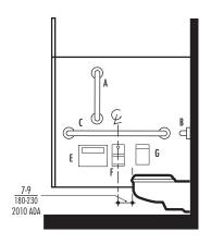
36 max 24 min 610 B C 18 min 455 1220 To top of outlet C: 14-19 355-485
