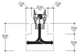
Fig. 2b T-Shaped Turning Space.
