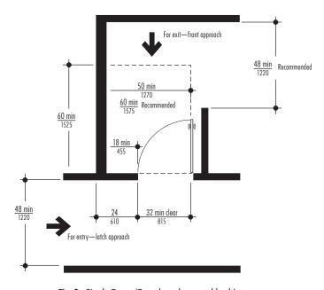
Fig. 3a Single Door. (Door has closer and latch)
