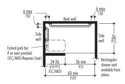
Fig. 24c Alternate Roll-In Type Shower Compartment (with seat).
