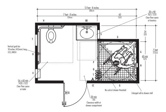
Fig. 30 Bathroom with Roll-in Shower Compartment.
