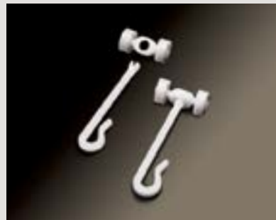
Breakaway Carrier 975P For use in psychiatric institutions. The hook is designed to pop out of the axle when 22 lbs of pressure is applied.
