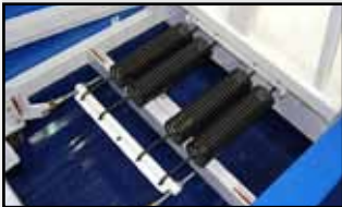
SPRING ASSIST OPERATION
